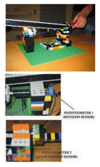
Fig. 6. The first prototype of the Croaker (left). Placement of the two potentiometers in the Croaker. The first potentiometer detects the position of the lever, while the second detects the position of the crank (right).
