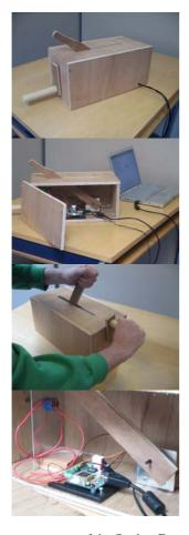
Fig. 8. The current prototype of the Croaker. From top to bottom: a view of the instrument, a view of the microcontroller and the sensors inside the instrument, use of the instrument and a close view of how the sensors are connected to the lever and crank.
